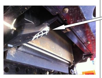
2. Trim plastic air dam using an air saw / multi
