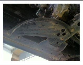
Remove and discard OEM shield from transfer case.
