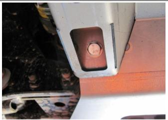
With the help of another person or a jack lift the transmission panel into place and secure the front section using 3 x Ø M8 x 25 bolts, flat washers and flange nuts.
